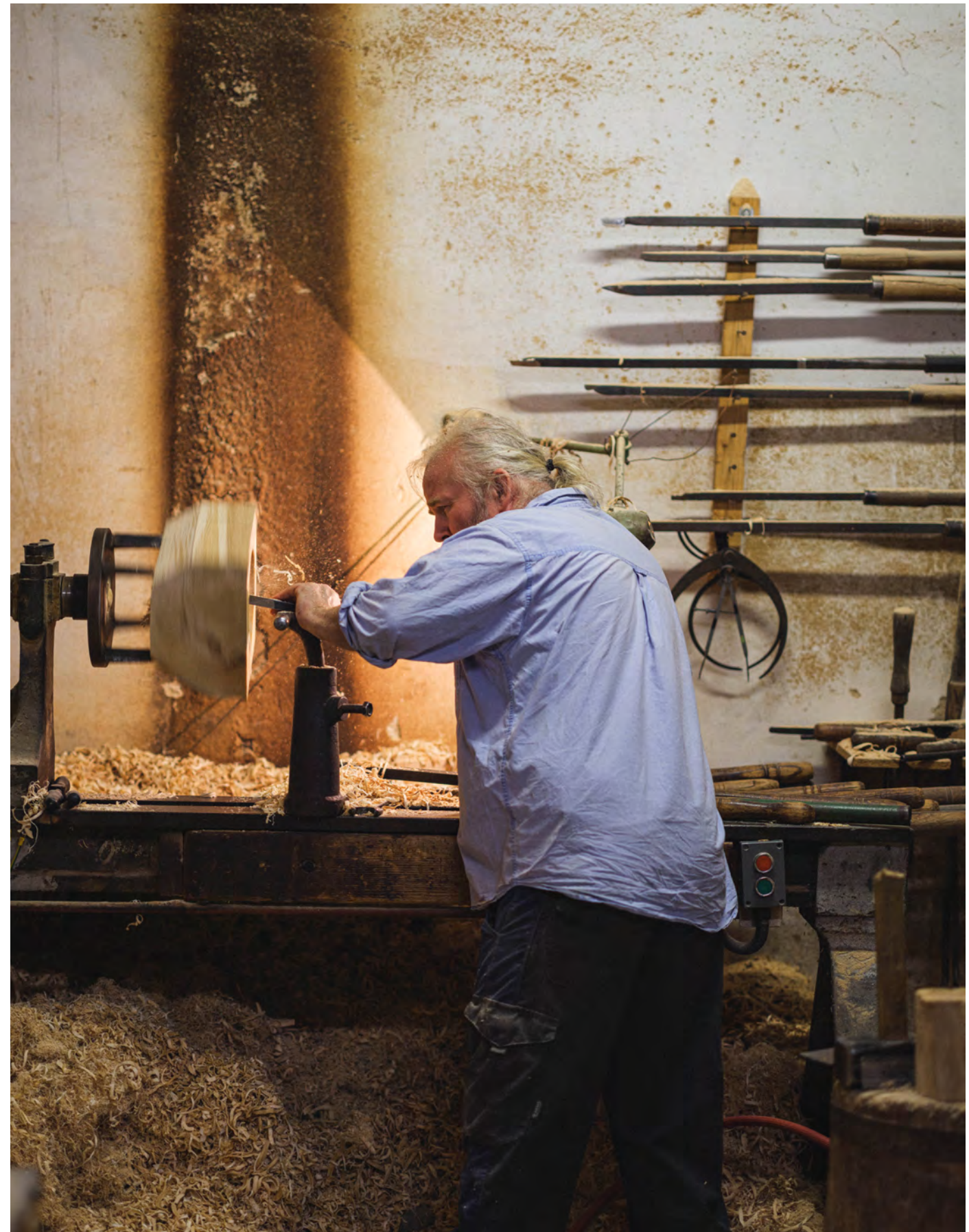
Creating a wooden mold.
